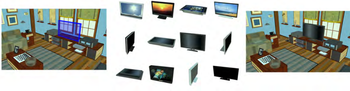
Figure 4.1: Scene modeling using a context search. Left: A user modeling a scene places the blue box in the scene and asks for models that belong at this location. Middle: Our algorithm selects models from the database that match the provided neighborhood. Right: The user selects a model from the list and it is inserted into the scene.
